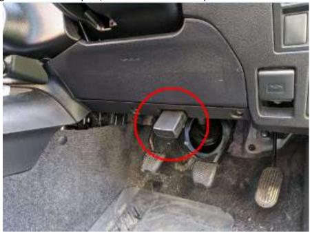
5. Remove the panel holding the OBDII connector and disconnect the OEM Connector. Example below, this was as simple as two screws and clips on the sides on the connector.
