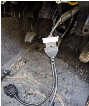
7. Fit the connector with the clips into the panel where the vehicle's established one was, and connect the OBD device into the smooth connector. Use the provided cable tie to secure the tracker onto existing wiring/harness or find a secure way to attach underneath column.
