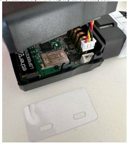
3. Once active, the GPS tracker PCB board will flash green, this indicates it is powered and ready to use. Close the black casing and install the sticker on the back surrounding the LED green light. The sticker will peel off and can be attached to the casing in the same direction:
