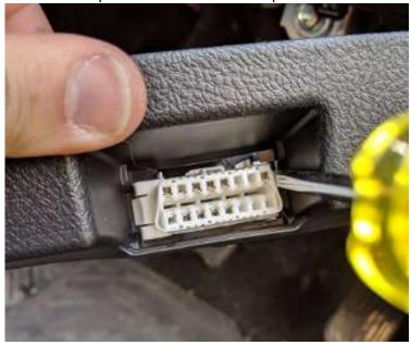
6. Connect the single connector end of the Splitter to the vehicle's established connector. The Cable is then tucked behind the panelling to hide it from view (discreet installation). Note: When concealing the OBDII splitter cable behind the panels, take care not to place the device or cables in a space that has been left empty intentionally to allow for the movement of parts such as steering wheels or pedals.
