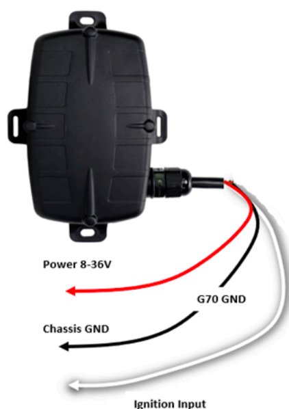
Standard 3 Wire Install Wiring Diagram
