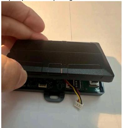
Step 3 - Connect small power clip to mainboard
